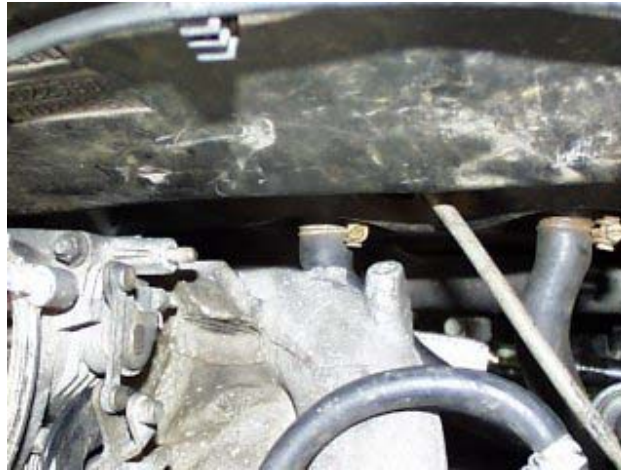
Inlet manifold gets in the way of the drivers side heater matrix pipe.
