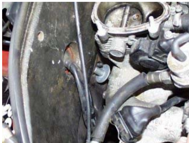
This is what happens when you don't modify the bulkhead. Make sure the clutch cable exits the bulkhead pointing towards the front passenger corner
