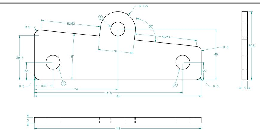
THREE OF THESE ARE NEEDED PER CONVERSION. THEY SHOULD BE USED WITH AN ANTI-CRUSH PIPE FOR THE THIRD BOLT, AS SHOWN BELOW:
