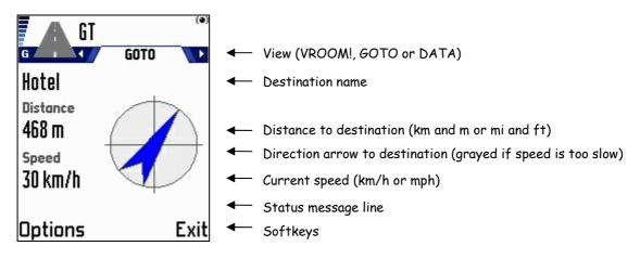
Navigation view (GOTO, see above) shows the name of the selected destination, the distance to it and the direction to it with a large arrow. It also shows the current speed. Note that the GPS receiver can determine direction only if you are moving (the arrow is grayed if the speed is below 2 km/h or 1.5 mph).
