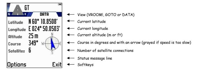
GPS data view (DATA, see above) shows the current latitude, longitude, altitude above mean sea level, course in degrees and with an arrow, and the number of GPS satellites being tracked.
